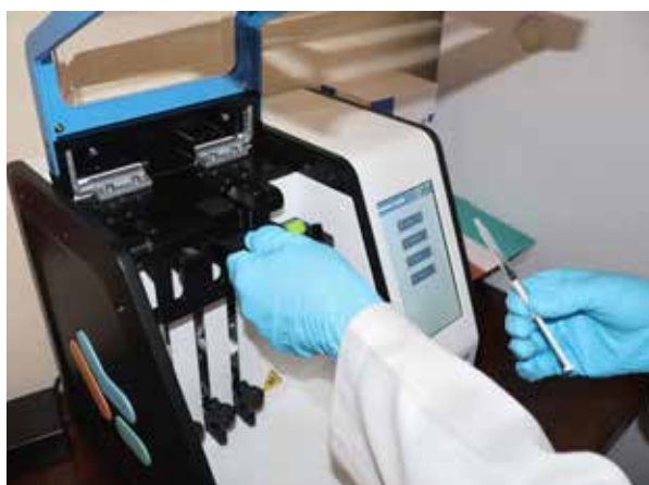
The microfluidics device, from Precision NanoSystems, is a vital piece of equipment in the Wits/SAMRC Antiviral Gene Therapy Research Unit. It is used to assemble mRNA-containing lipid nanoparticles (LNPs) for application as vaccines and therapies.
